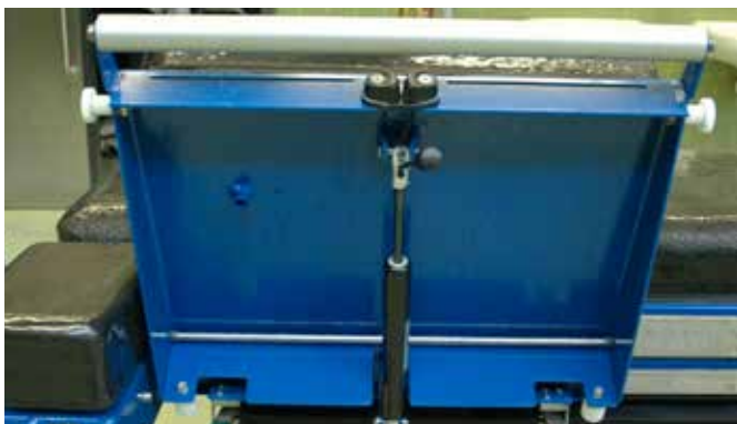
Side panels is stepless controlled by gas hydraulic cylinders
