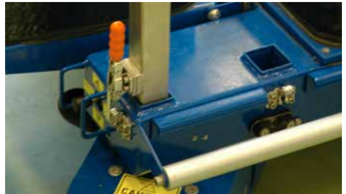
Vertical bars for leg support are locked to frame - cannot be accidentally pushed out
