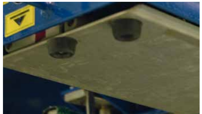
Safety switch under each corner & head support - no leg injury when lowering the table
