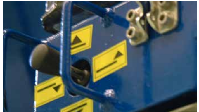
Joystick in each corner controls lift and tilt - no need for remote control
