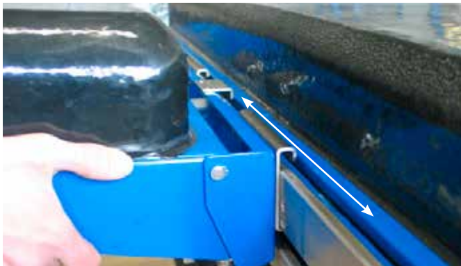
Side panels can easily be removed or moved
