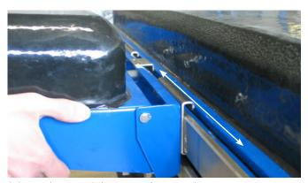
Side panels can easily be removed or moved
