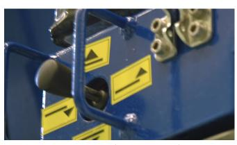
Joystick in each corner controls lift and tilt - no need for remote control
